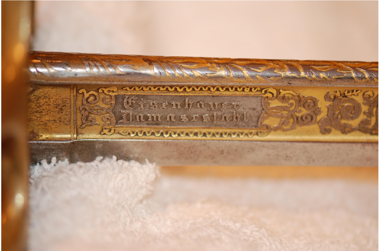
“Eisenhauer” and “Damaststahl” on the opposite side of the decorated blade, identify both the Solingen bladesmith and the quality of the steel manufactured
